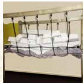
According to DIN EN 1176-1, a safety factor of 1.35 is mathematically required, in practical proof a factor of 2.
